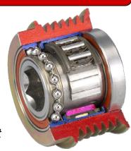
The benefits of this type of pulley system are more readily seen on vehicles that have rapid speed changes as well as high alternator loads. Systems using these types of pulleys have less belt noise (no chirping during speed changes) and smoother idle operation. This type of belt drive system has been popular in the heavy truck industry on diesel and odd cylinder engines in Europe.
